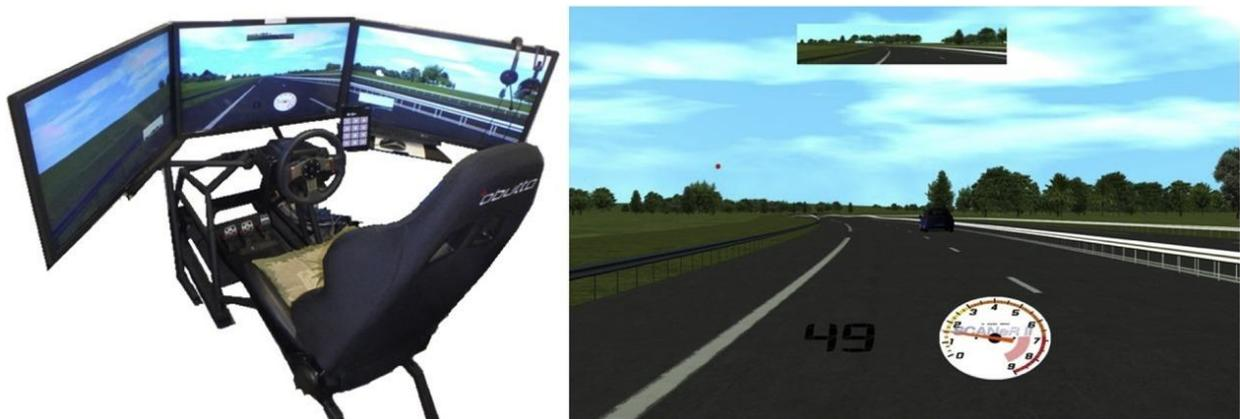
*Note.* The left panel shows the driving simulator with the tablet device positioned next to the steering wheel. The right panel shows the central monitor view of the driving environment with rear-view mirror and digital speedometer displayed.<sup>1</sup>
